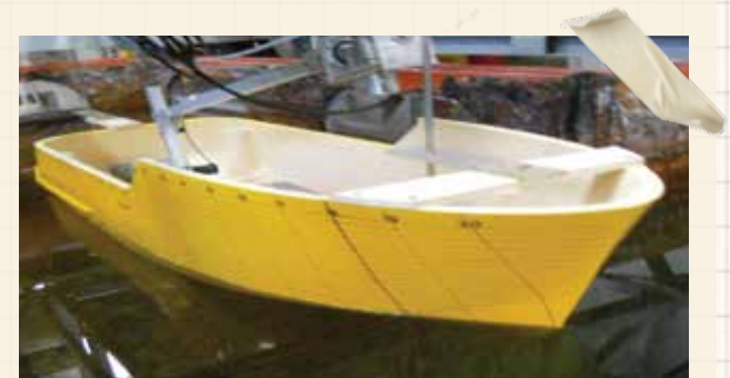
Ocean King model in a ship model basin
