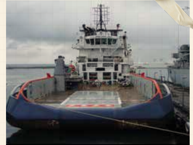
"Open Stern" in a real Explorer
