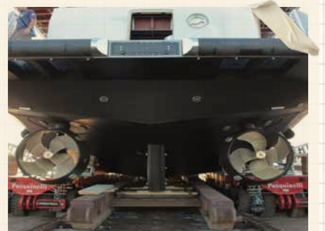
Propellers in the Ocean King are protected by skeg to avoid accidental injury with submerged objects
