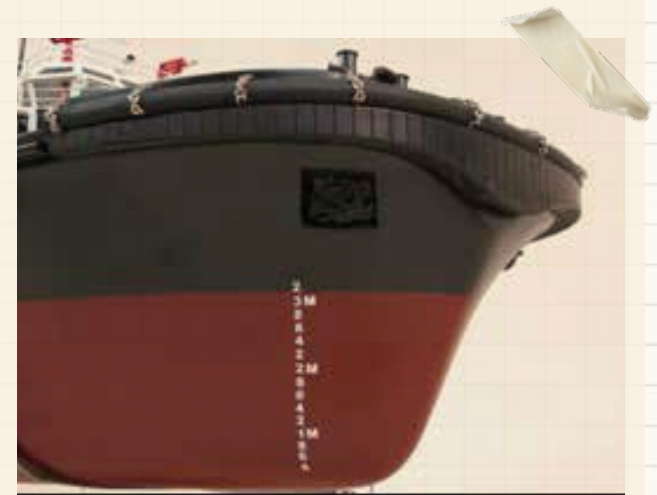
Bows of “true tugs”, without bulb bow like on Ocean King
