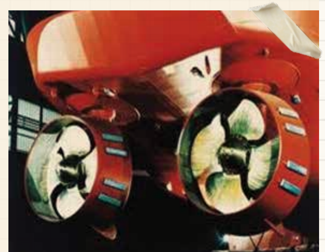
Propellers with Azimuth transmission
