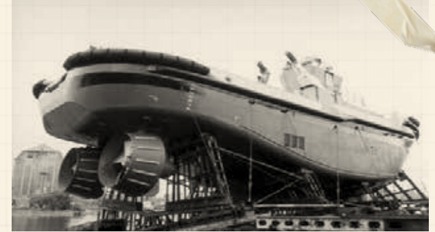
A real hard chines hull in a real Tug, the same hull of Ocean King
