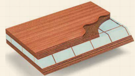
A sandwich panel for acoustic and thermal insulation
