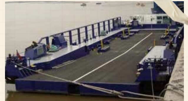
Hard chines hull used on Ocean King
